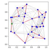
For each TSP, *n* node locations sampled randomly in the unit square. Optimal tour found using Concorde.
