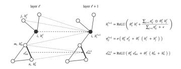
Final *h*-dimensional embedding  $e'_{ij}$  for each edge is fed to a Multi-layer Perceptron classifier to compute the probability of that edge being connected in the TSP tour.
